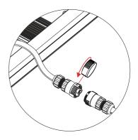
Connect the light with power source Turn the knob to the bottom.
