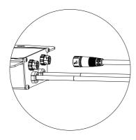
Connect the dimming wire and the power core together, and twist it until it's tight.
